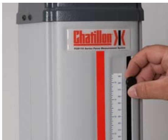
Shown: Mechanical travel limits are located on the front of the column. A reference rule is supplied that allows you to accurately locate your maximum travel limits.
