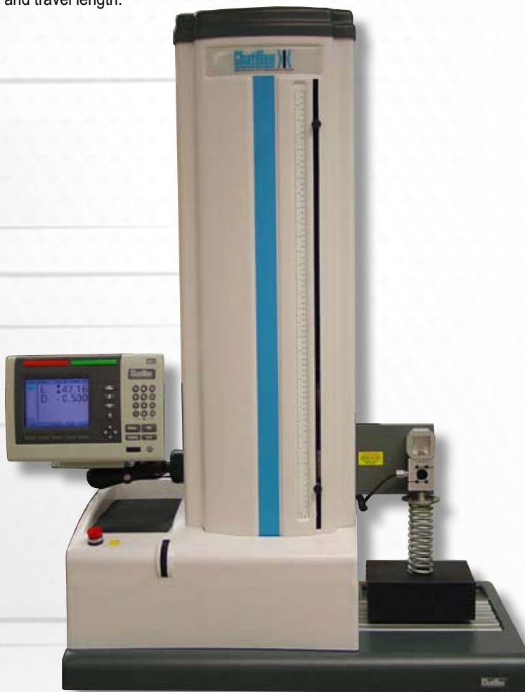
TCD1100 System shown testing an automotive spring.
