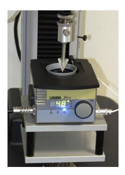
Penetration test with peltier system able to generate temperature from 5°C to 80°C.
