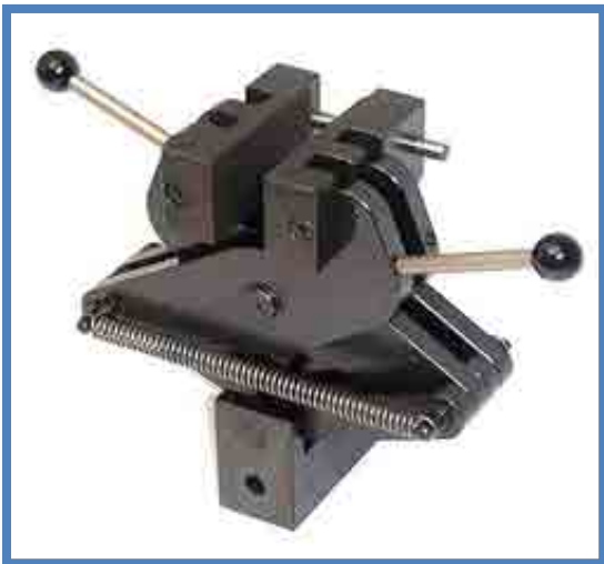
01/4213 Crosscut Face 1.2 x 45° Pitch Hardened Steel 58HRC Nickel Plated
