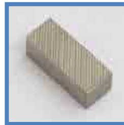
Crosscut Jaws 0.8 x 45° crosscut Hardened 58HRC
