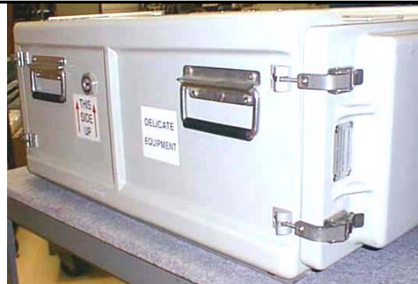
MPCU with covers in place; handles and pressure relief valve can be seen
