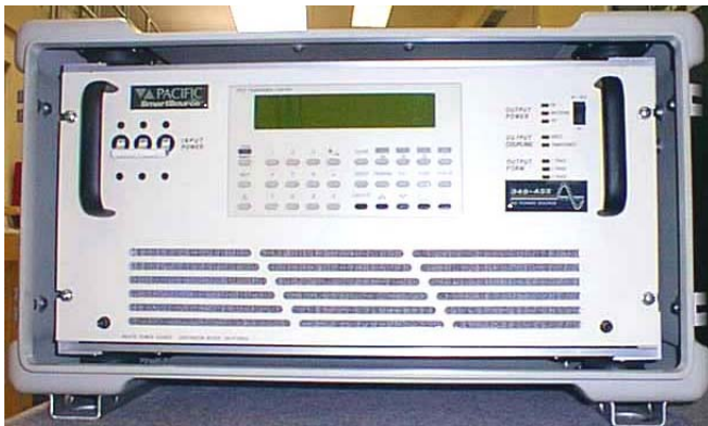
MPCU with Front Cover removed showing 345ASX-UPC3 front panel
