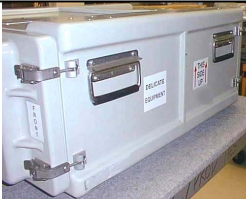
MPCU with covers in place; handles and pressure relief valve can be seen
