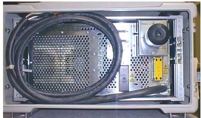
MPCU with rear cover removed showing rear 400Hz output receptacle on the 345ASX-UPC3 and input power cable
