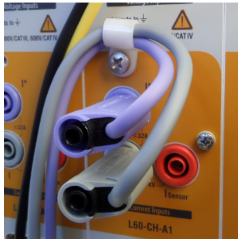
Figure 3.24: screw mounted cable clamps
