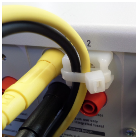
Figure 3.25: screw mounted cable tie mounts
