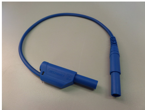
Figure 3.13: Safety laboratory lead for general purpose
