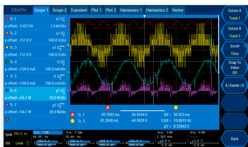
Simultaneous measurement of narrowband and wideband values
