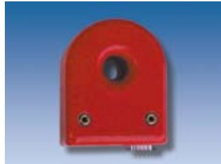
PSU600 Precision current transformer, max. 600A, \bar{u}=1500:1 , DC to >100kHz, accuracy <(0.01%MV+0.005%MR)
